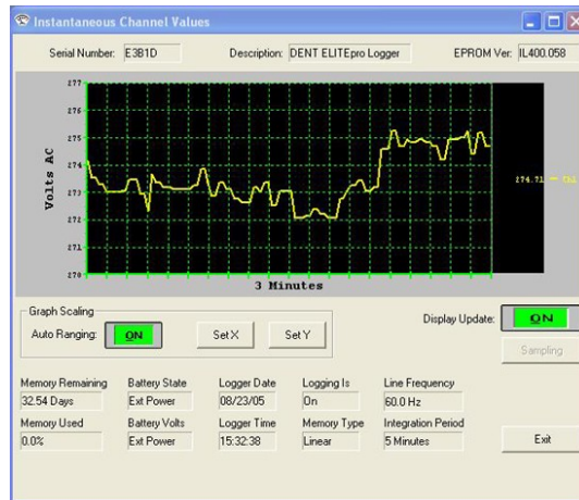
Instantaneous Channel Values: See information about your logger and what your logger is recording in real time.
