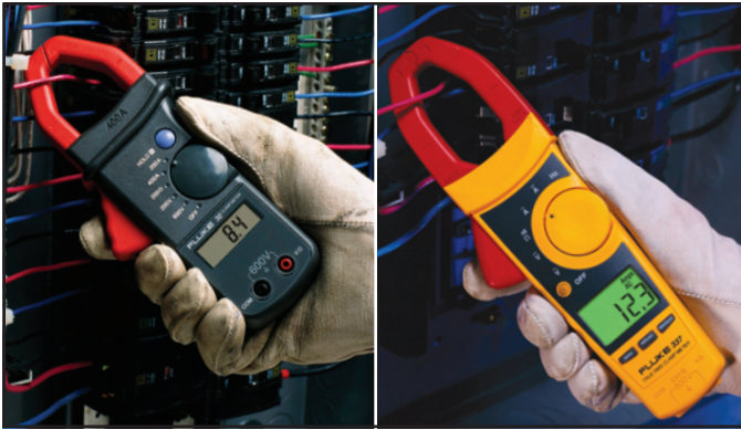
One current—two readings. Which do you trust? The branch circuit above feeds a non-linear load with distorted current. The true-rms clamp on the right reads correctly but the average responding clamp reads low by 32 percent.
